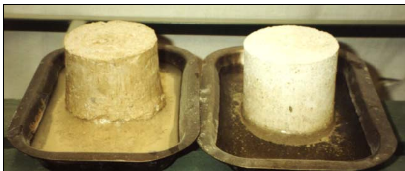
Figure 5 A view of a pavement material sample unstabilised (left) and stabilised with DPP (right) subject to soaking in water for 24 hours.
